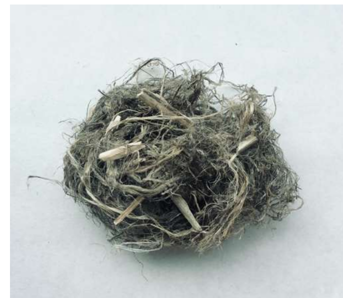
Figure 1 - Technical grade hemp fibres
