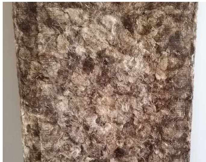
Figure 3 - Self-supporting wool/hemp insulation board
